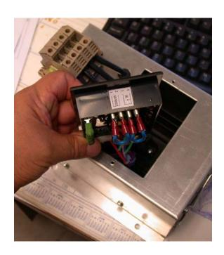
Changing the U/F set point by removing the jumper in the controler. ON for 60 OFF for 50Hz. You can also add a 1K Ohm 1/2 wire resistor for remote voltage adjustment.
